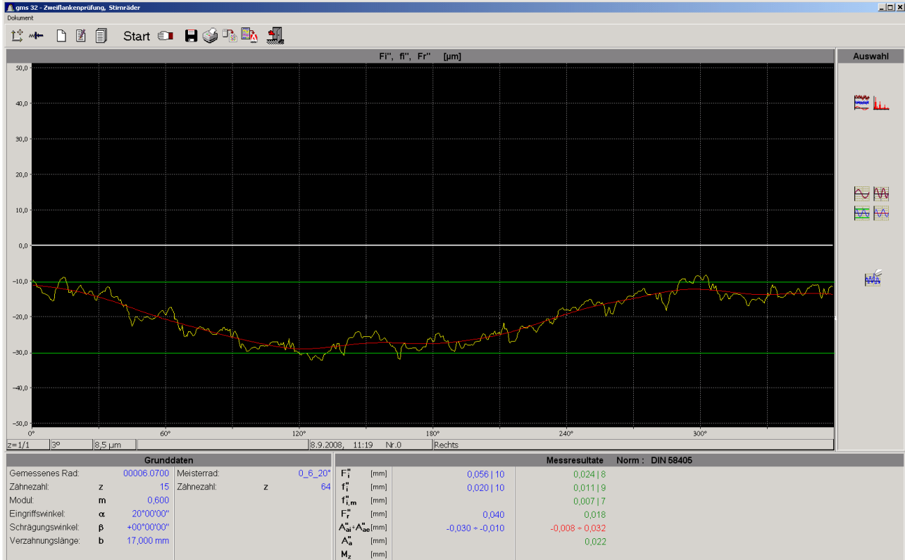
Figure 5- Example diagram of a gear with tooth backlash
