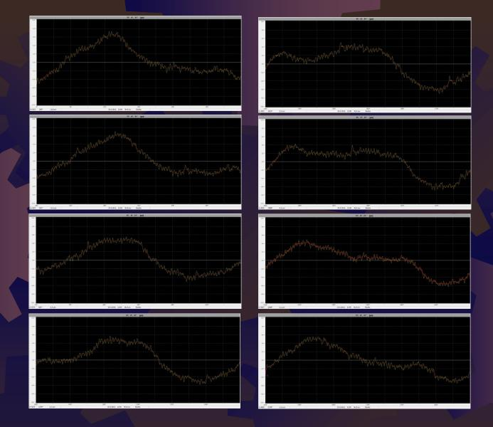
Why is each revolution different? It is caused by the master gear error.
